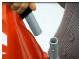
10. Slide the clamp back onto the bottom of the pole and tighten it.
